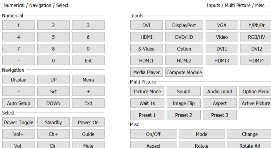
Select the display to control from the **Apply To Display** list. Click the buttons to send the IR Remote command to the display. The display will respond as if it received a signal from the IR Remote control.
