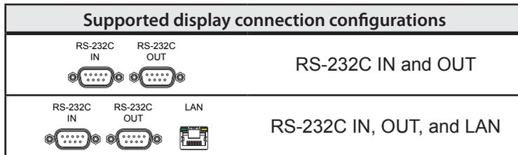
Models that have two RS232 connections (not including any RS232 connections on OPS devices), support RS232 daisy-chaining. The connection labeled IN is the input to the display from the host PC. The other connection labeled OUT is the output to connect to the IN on the next display in the daisy chain.
