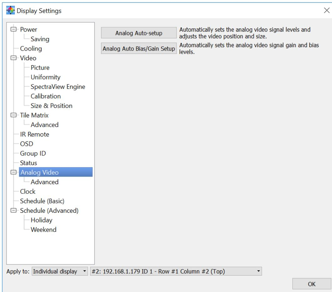
The **Analog Video** panel can be used to set special video adjustment patterns to assist with manual adjustment of the analog video input levels.
