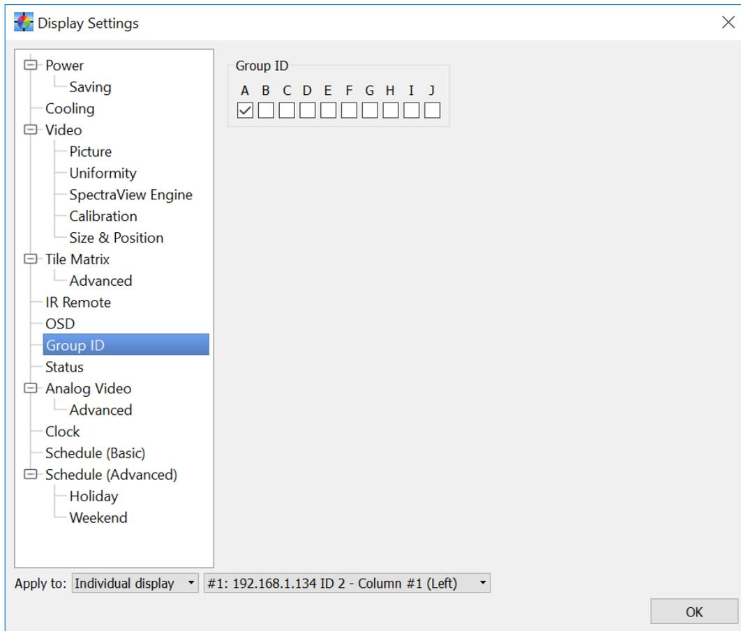
The **Group ID** panel is used to assign the selected monitor(s) to different addressable logical groups. Group IDs can be used to address multiple displays via control commands addressed to individual groups. *NEC Display Wall Calibrator* does not use the Group ID but other applications can make use of this functionality.
