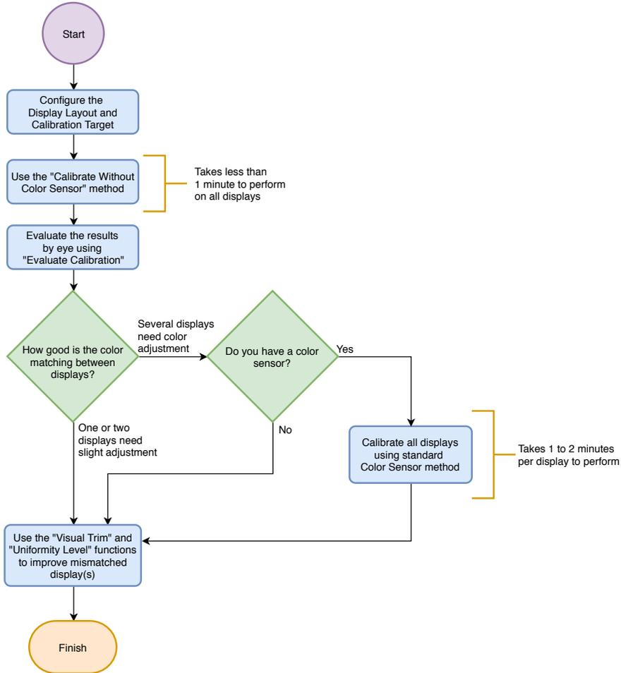
Figure 3: Overall calibration determination for displays and analog video inputs
