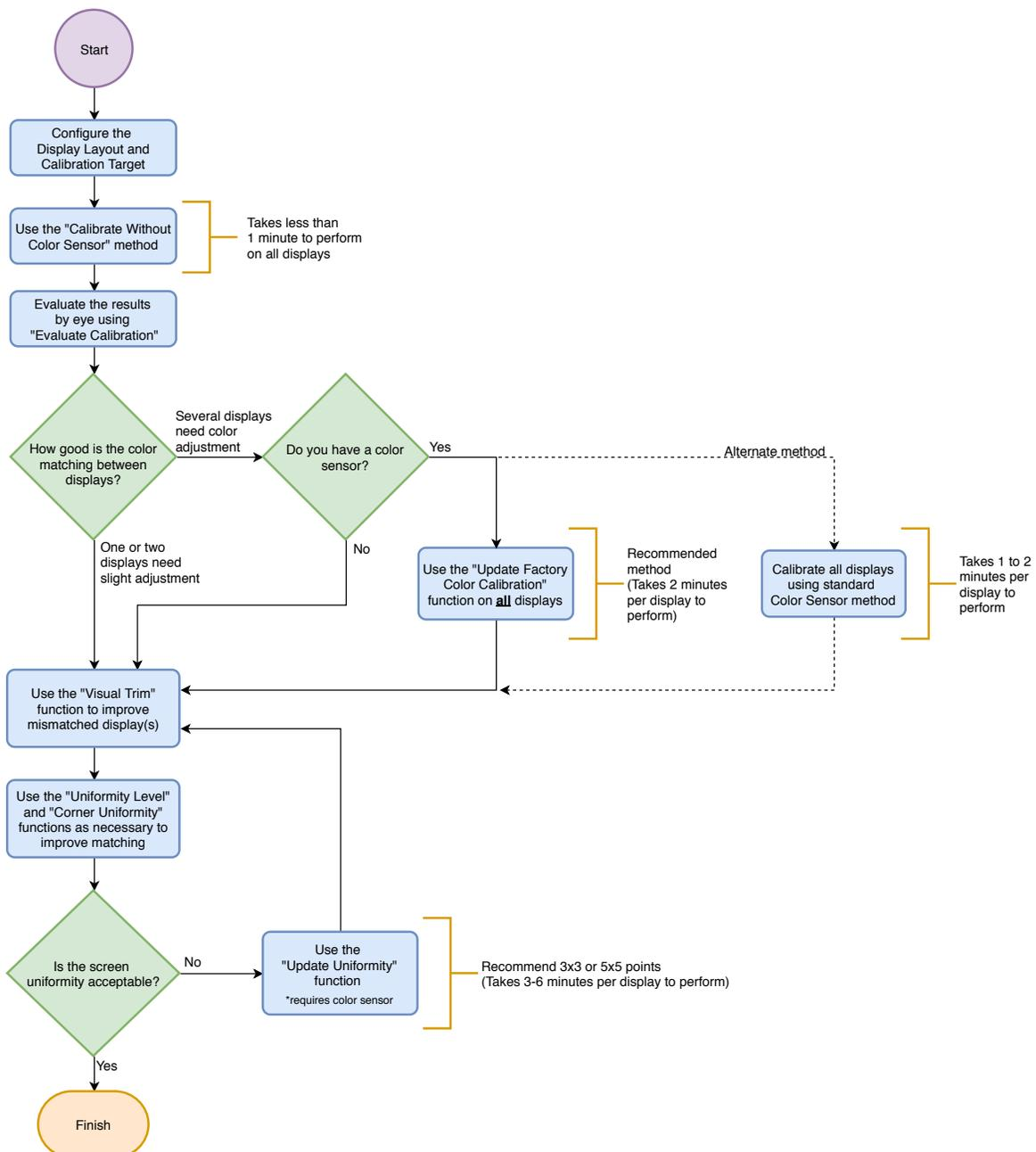
Figure 2: Recommended calibration procedure for SpectraView Engine models
