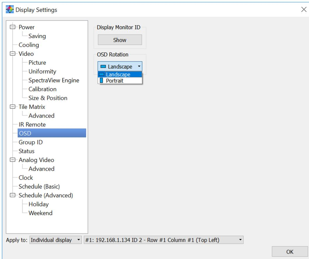
The **OSD** panel can be used to show the display's monitor ID and rotate the OSD menu.
