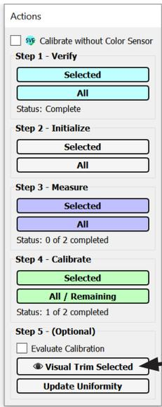
Once a display has been calibrated, the *Evaluate Calibration* checkbox and the *Visual Trim* button will be enabled in the *Actions* panel.
