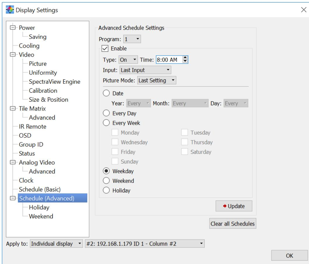
The **Schedule (Advanced)** panel is used to set the schedule function in the display. Various scheduled operations such as power on, power off, and changing inputs can be configured.
