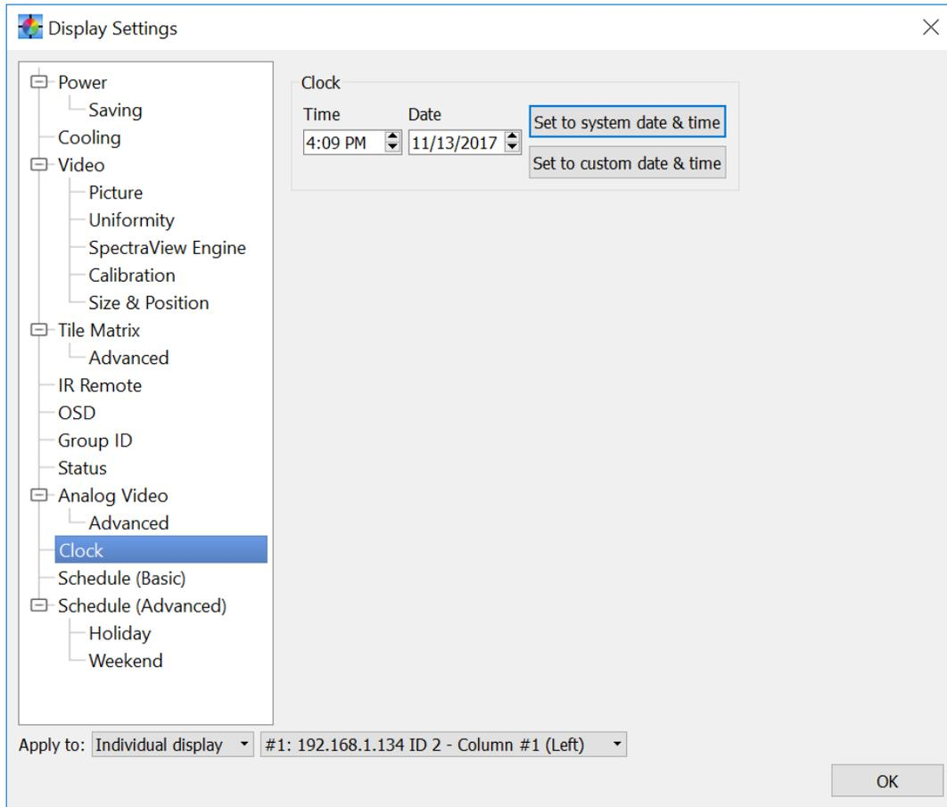
The **Clock** panel is used to set the internal real time clock and schedule functions in the display. Various scheduled operations such as power on, power off, and changing inputs can be configured.
