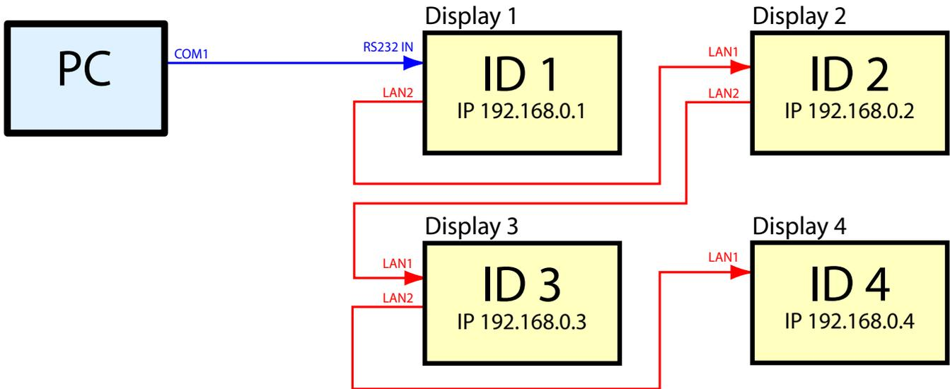
The first display will translate and forward RS232 communications from the host PC over the LAN connection to the other displays.
