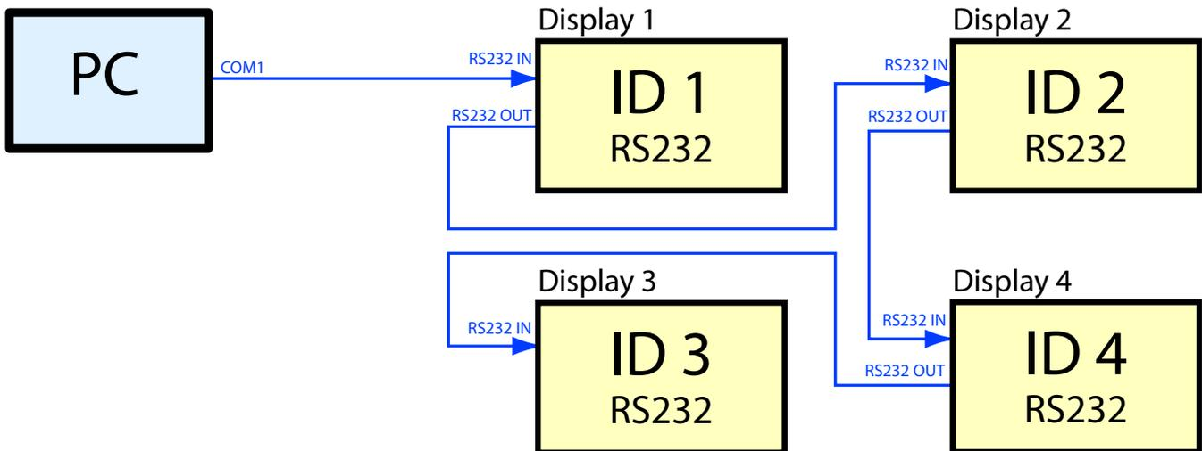
**Info:** For RS232 daisy-chains, the cable connections between displays does not need to follow the same ordering as the ID assignments. In this example the daisy-chain is connected in order 1 - 2 - 4 - 3.
