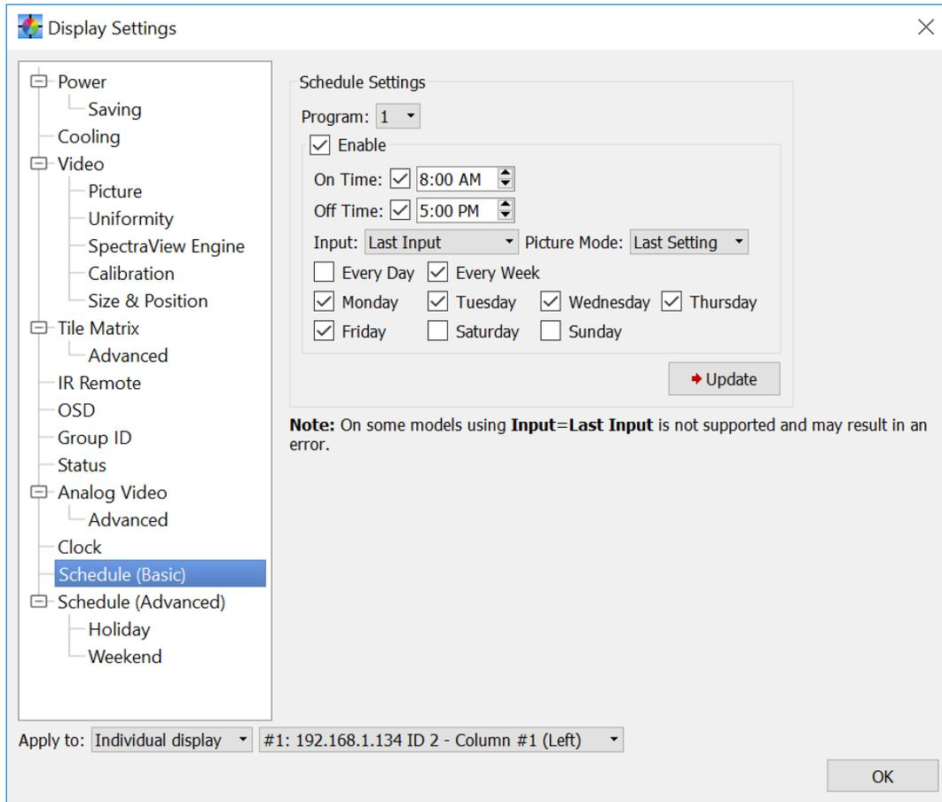
The **Schedule (Basic)** panel is used to set the schedule function in the display. Various scheduled operations such as power on, power off, and changing inputs can be configured.
