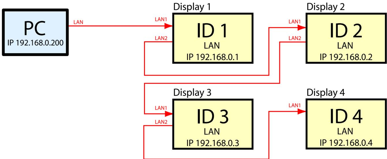
The displays act as 2-port LAN hubs and pass LAN communications through.
