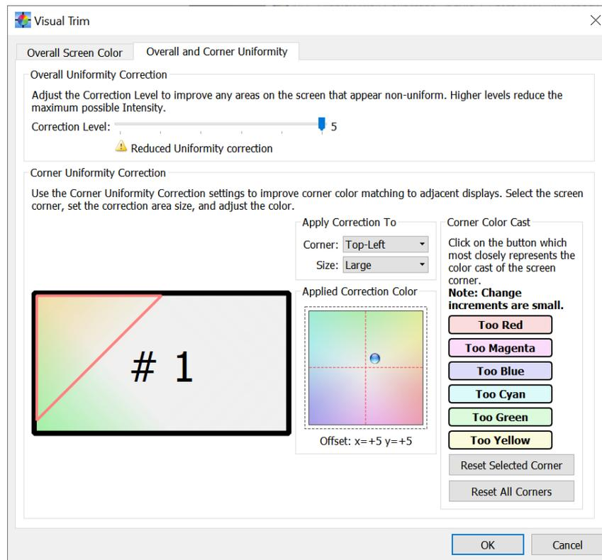
Use the **Uniformity Correction** slider to adjust the Correction Level to improve any areas on the screen that appear non-uniform. The lowest setting disables the Uniformity Correction entirely. Level 1 reduces any color unevenness across the screen but with the trade-off of reduced luminance evenness, especially around the edges of the screen. Higher levels of correction improve the luminance evenness across the screen, including around the edges.
