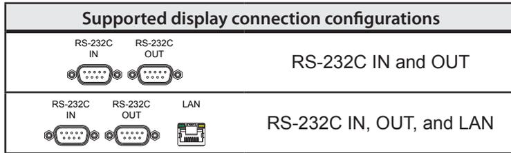
In this example, the host PC has one RS232 COM port and all displays are daisy-chained together via RS232. Each display must have a unique MONITOR ID since they are all on the same daisy-chain. The RS232 OUT on the first display is connected to the RS232 IN on the next, etc.
