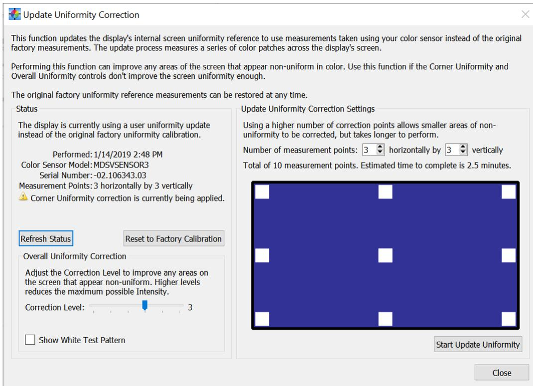
For display models that include the SVE and screen Uniformity Correction feature, each display was individually analyzed during factory production to measure the color and luminance uniformity across the entire screen. These measurements are stored in the display, and the SVE can create a Uniformity Correction to even out the screen uniformity.
