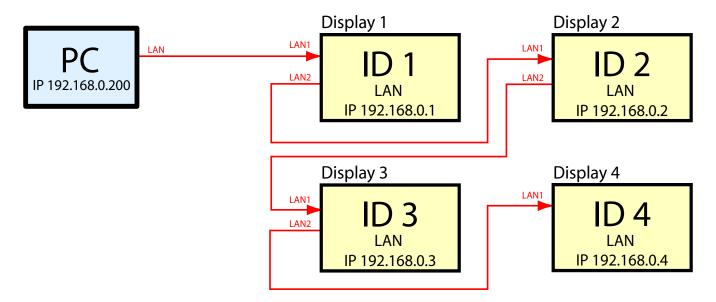
The displays act as 2-port LAN hubs and pass LAN communications through.
