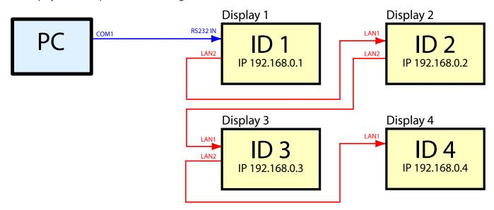
The first display will translate and forward RS232 communications from the host PC over the LAN connection to the other displays.
