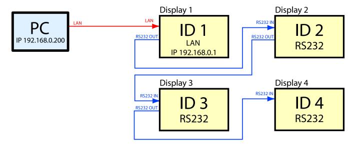
The following image shows how this layout looks in the Summary window when configured. Notice that all of the displays are configured in the software to use the LAN IP address 192.168.0.1, even though displays 2, 3, and 4 are connected together via RS232.
