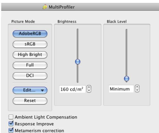
The **Picture Mode** panel controls the settings for the various Picture Modes that the monitor supports, and is also used for adjusting the Brightness and Black Level.
