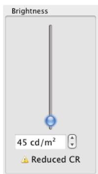
“Reduced CR” is shown when the Brightness control is set to a level where it impacts the Contrast Ratio of the screen image. This occurs when the brightness setting is below that which can be controlled using the LCD backlights alone.
