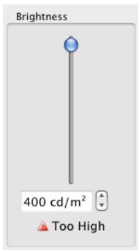
"Too High" is shown when the Brightness level setting is too high and cannot be achieved by the monitor with the current setting. Lower the setting until the message disappears. It takes several seconds to update the level warning.
