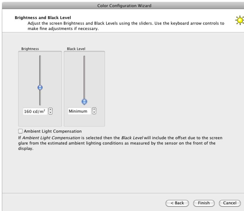
The **Brightness** slider and spinbox controls adjust the monitor brightness. The brightness is indicated in Candelas per square meter ( $\text{cd/m}^2$ ) on display models that have an internal luminance sensor and represents an absolute value.
