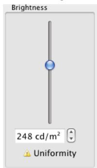
“Uniformity” is shown when the Brightness control is set above the range that the monitor can achieve with the current Digital Uniformity Compensation setting.
