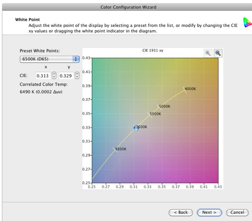
The white point of the monitor can be altered using the wizard by either clicking and dragging the positioning control on the CIE xy diagram or modifying the **CIE x** and **y** values.
