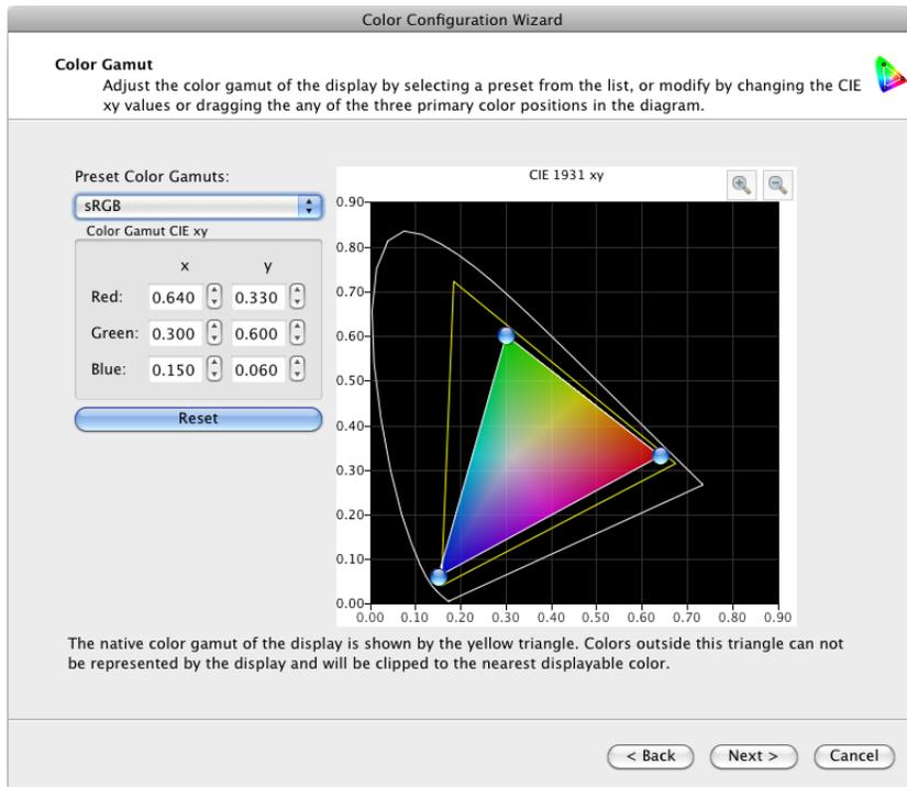
The color gamut is the range of colors that can be displayed by the monitor. The color gamut of a monitor is defined and bounded by the red, green, and blue primaries which together make up all other colors. The SpectraView Engine is capable of manipulating these primary colors in order to display different colorspace.
